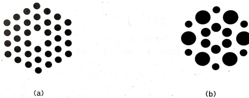
Fig: Two index guided photonic crystal fibers .The dark areas are air holes and white areas are silica.
